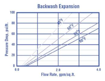
**Backwash:** After each cycle the resin bed should be backwashed at a rate that expands the bed 50 to 75 percent. That will remove any foreign matter and reclassify the bed.
