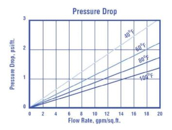
**Pressure Drop:** The graph above shows the expected pressure loss per foot of bed depth as a function of flow rate at various Temperatures.
