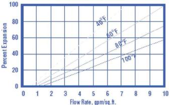
**Backwash:** After each cycle the resin bed should be backwashed at a rate that expands. The bed 50 to 75 percent. That will remove any foreign matter and reclassify the bed. The Graph above shows the expansion characteristics of G-ion GC 100 in the sodium form.
