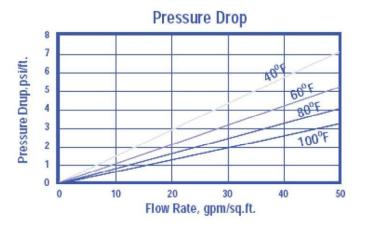
**Pressure Drop:** The graph above shows the expected pressure loss per foot of bed depth as a function of flow rate at various Temperatures.
